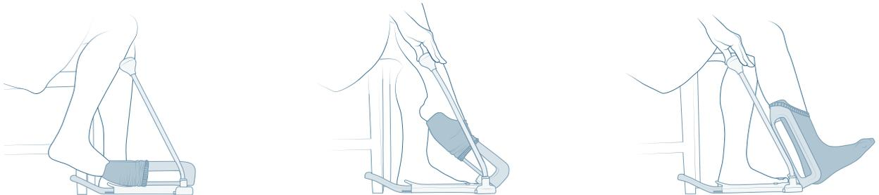
While sitting comfortably upright on the chair, move the Sockee arm with your leg to face the outer side of the chair. Pull your leg back slightly around the outer side of the chair, and slide your foot into the sock. As your heel reaches the edge of the Sockee arm, raise your foot slightly then push down while flexing your foot. (in case you are using long socks, finalize the action by pulling the socks up with your hands). Repeat steps 3-8 to put on your other sock.
