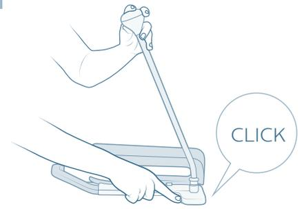
Attach the handle to the base by pressing the button, until it clicks. The Sockee device is now ready for use.
